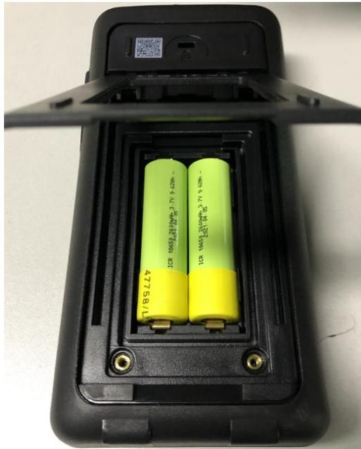
Figure 4.9 Install the battery
