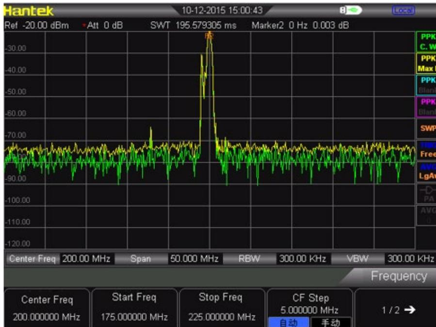
6. Press [AMPT] → Attenuation → 10dB to turn up the RF attenuation to 10 dB.
